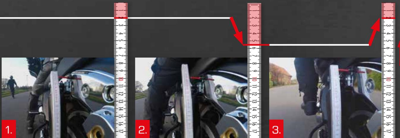
Vehicle in defined level position after the driver has climbed on.
